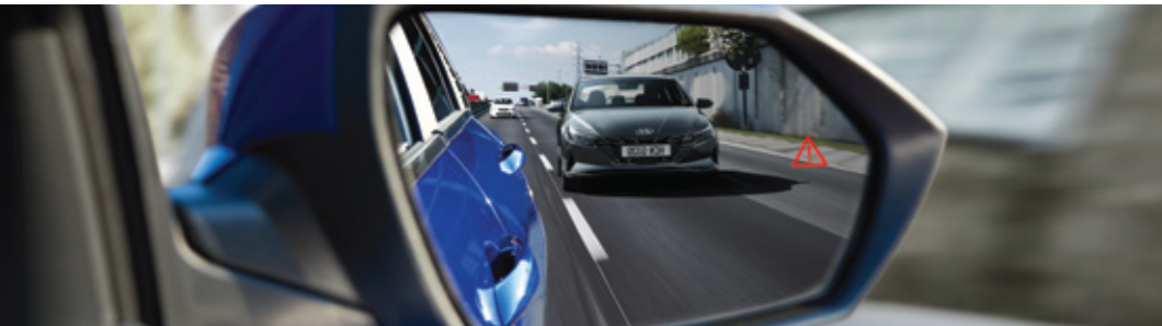
Blind-Spot Collision-Avoidance Assist (BCA) When operating the turn signal switch to change lanes, if there is a risk of collision with a rear side vehicle, it provides a warning. After the warning, if the risk of collision increases, it automatically controls the vehicle to help avoid a collision.
