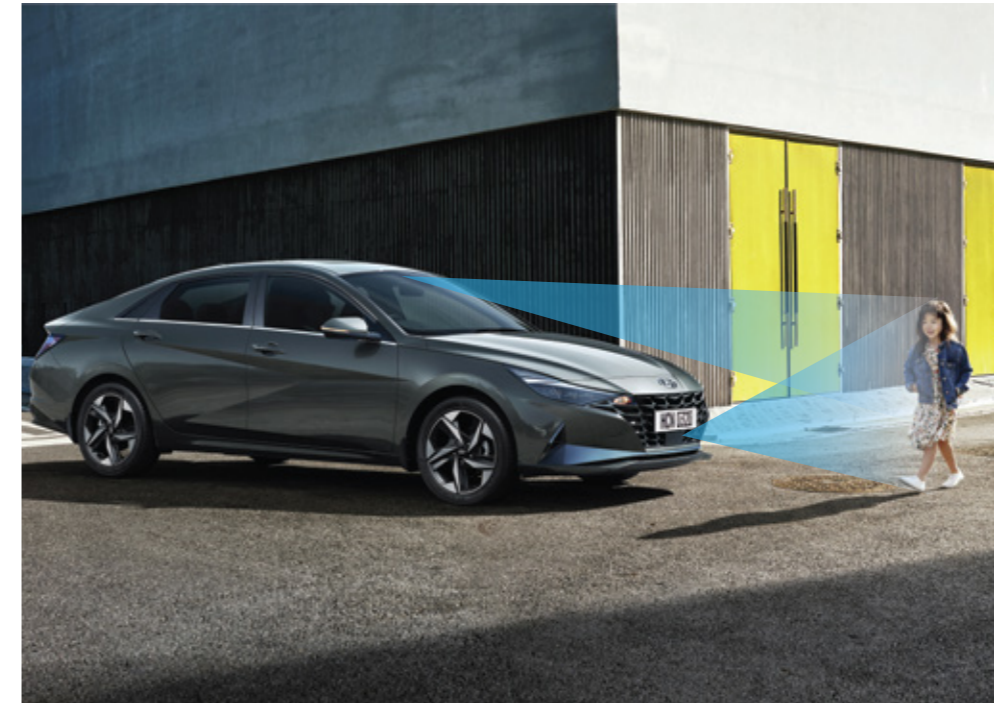
Forward Collision-Avoidance Assist (FCA) If the preceding vehicle suddenly slows down, or if a forward collision risk is detected, such as a stopped vehicle or a pedestrian in front, it provides a warning. After the warning, if the risk of collision increases, it automatically assists with emergency braking. While driving, if there is a risk of collision with a cyclist, it automatically assists with emergency braking. If there is a risk of collision with an oncoming vehicle while turning right at an intersection, it automatically assists with emergency braking.
