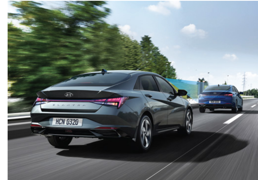
Smart Cruise Control (SCC) with Stop & Go Smart Cruise Control helps maintain distance from the vehicle ahead and drive at a speed, set by the driver. The vehicle stops automatically and starts automatically if the vehicle in front starts in a short time. If a period of time has elapsed, start again by pressing the accelerator pedal or operating the switch.
